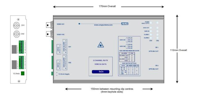
The **AMG5625** is a **DUAL** rackmount system which provides two independent channels, each designed to transmit 1 video signals plus 2 Uni-directional alarms and transmit and receive 1 data signal over one Multimode optical fibre.
